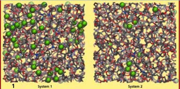
1 Structure models of two different UV-curing clearcoats with non-crosslinked double bonds.
